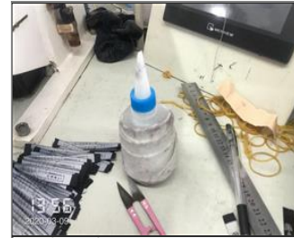
Photo of non-conformity NC chemical without label.JPG
